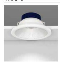
**Technical:** 22W TRIDONIC LED | 2000Lm | CRI 80 | 3000K, 4000K | Tridonic Control Gear | 220-240V | IP20
