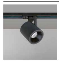
**Technical:** 12W LUMINUS LED | 900Lm | CRI 90 | 36° |3000K | Included Control Gear | 220-240V | IP20
