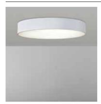
Technical: 38W / 51W TRIDONIC LED | 5880Lm / 7900Lm | CRI 80 | 3000K, 4000K, 6000K | Tridonic Control Gear | 220-240V | IP20
