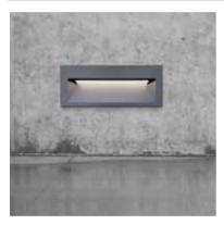
**Technical:** 4W LED | 240Lm (Light source) 120Lm (Luminaire) | CRI 80 | 3000K, 4000K, 6000K | Included Control Gear | 220-240V
