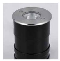
Technical: 8W LED CREE | 683Lm (light source) 473Lm (Luminiare) | CRI 85 | 15°, 24°, 36° | 3000K-6000K | HEP Control Gear | 100-240V | IP67
