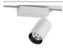
**Technical:** 37W LED Lumileds | 4625Lm (light source) 3890Lm (luminaire) | CRI 90 | 25°, 35°, 45° | 2700K, 3000K, 4000K | Osram Control Gear | 220-240V | IP20
