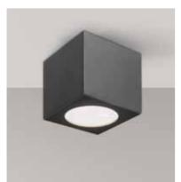
**Technical:** 6W LED | 420Lm | CRI 80 | 3000K | Included Control Gear | 220-240V | IP54
