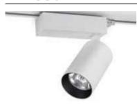
**Technical:** 31W LED Lumileds | 4000Lm (light source) 3350Lm (luminaire) | CRI 90 | 25°, 35°, 45° | 2700K, 3000K, 4000K | Osram Control Gear | 220-240V | IP20
