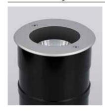
**Technical:** 16W LED CREE | 1083Lm (light source) 975Lm (Luminiare) | CRI 85 | 15°, 24°, 36° | 3000K-6000K | HEP Control Gear | 100-240V | IP67
