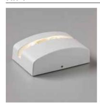
**Technical:** 5W LED Philips | 450Lm (light source) 200Lm (Luminiare) | CRI 80 | 3000K | Included Control Gear| 220-240V | IP65
