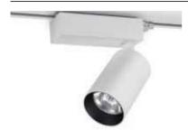
**Technical:** 24W LED Lumileds | 3000Lm (light source) 2510Lm (luminaire) | CRI 90 | 25°, 35°, 45° | 2700K, 3000K, 4000K | Osram Control Gear | 220-240V | IP20
