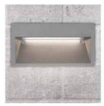
**Technical:** 10W LED | 600Lm (Light source) 400Lm (Luminaire) | CRI 80 | 3000K, 4000K, 6000K | Tridonic Control Gear | 220-240V | IP54
