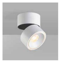
Technical: 14W LED Bridgelux | 1354Lm (light source) 992Lm (luminaire) | CRI 80 | 24°, 36° | 3000K | HEP Control Gear | 220-240V | IP20
