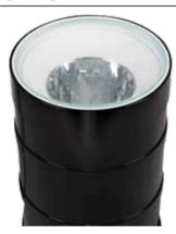
Technical: 16W LED CREE | 1083Lm (light source) 802Lm (Luminiare) | CRI 85 | 15°, 24°, 36° | 3000K-6000K | HEP Control Gear | 100-240V | IP67
