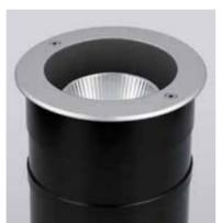
**Technical:** 22W LED CREE | 1555Lm (light source) 1010Lm (Luminiare) | CRI 85 | 15°, 24°, 36° | 3000K-6000K | HEP Control Gear | 100-277V | IP67
